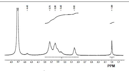
Figure 2. H<sup>1</sup>-NMR spectra of the initial chitosan ChS-1
