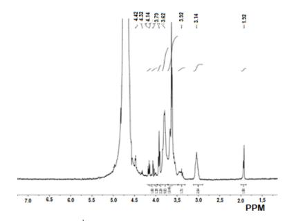
Figure 4. H<sup>1</sup>-NMR spectra of chitosan oligoascorbate ChSA-2
