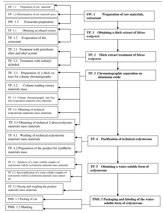
Figure 1. Technological scheme for the production of a water-soluble form of ecdysterone
